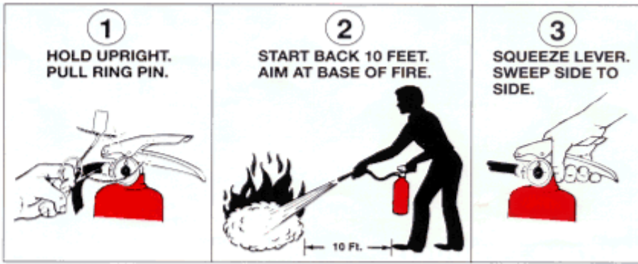
Fig: Steps to use fire extinguisher
