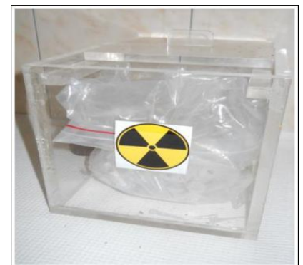
Fig: Waste disposal box
