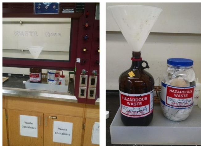
Fig: Disposal containers of hazardous waste
